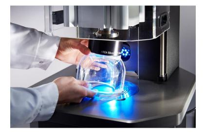
With the test dome removed, the stainless steel clamp ring can be removed by pressing with your thumb on the top surface close to the outer edge. The clamp ring will lift up at the opposite edge.
