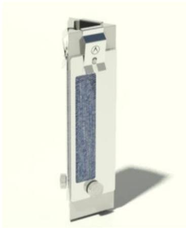
Finally lower the clips down to securely attach the specimen mask to the main body of the sample holder.
