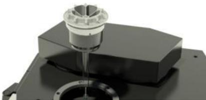
Ensure that the lamp is carefully lowered so as not to cause any damage to either the Xenon lamp or the KG1 filters inside the Lantern.
