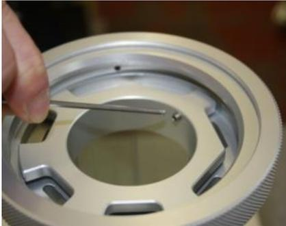
Finally, use a 2mm A/F Allen Key to secure the Allen Screw (See Picture).
