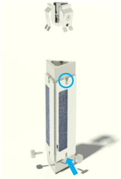
Next fit the specimen masks to the main body of the specimen holder.
