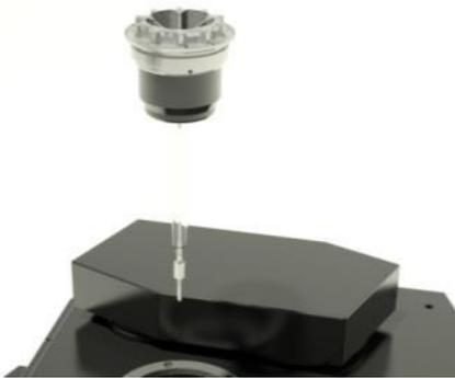
Once fully inserted, lower the Lamp Connector back into position.
