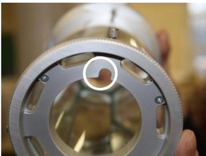
To position the Lantern inside the TruFade chamber find the location notch (highlighted by the white circle) on the Bottom End Cap.
