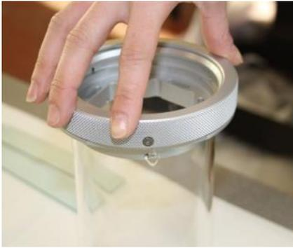
Now carefully lower the Top End Cap (largest End Cap) onto the Borosilicate Cylinder.
