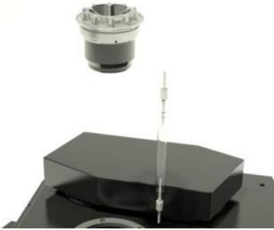
Remove the old lamp (if applicable) & Insert the new Xenon Lamp in to the Lamp Connector.
