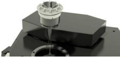
Replace the Xenon Lamp and secure the lamp connector by turning it clockwise until it cannot be turned further.
