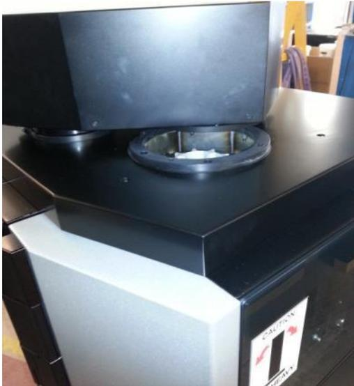
Once the air outlet is attached, swing the lid to the left until it clicks over the lamp access point.
