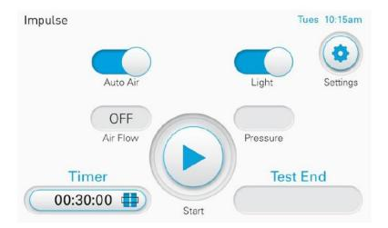
The air flow will not start until the test has begun, which is why the display window still shows as off. Once the test has started, the air flow comes on and the display window will change to ON.
